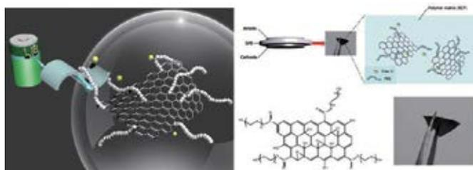
Polymer composite electrolytes having functionalized graphene oxide filler
