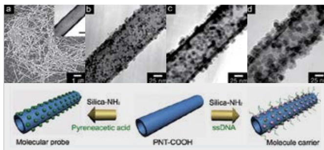
Fabrication of polypyrrole nanotube for molecular probe and DNA carrier applications
